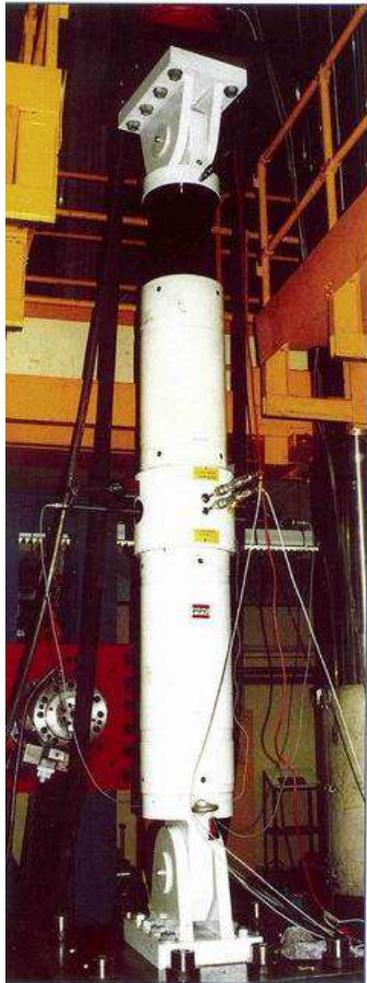
100 kN, 710 mm stroke Transpec® SHA damper.
