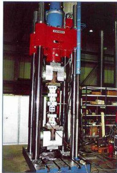
500 kN, 90 mm stroke Transpec® SHA damper.
